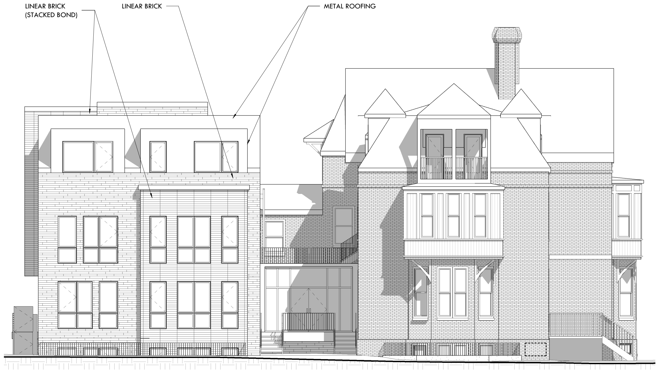
SD ELEVATION - WEST MATERIALS
